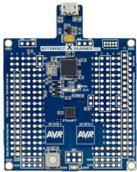
The ATtiny817 Xplained Mini Evaluation Kit (ATTINY817-XMINI) is a hardware platform for evaluating ATtiny817, ATtiny816, ATtiny814 and ATtiny417 microcontrollers. The evaluation kit comes with a fully integrated debugger that provides seamless integration with Atmel START and Atmel Studio development environment.
