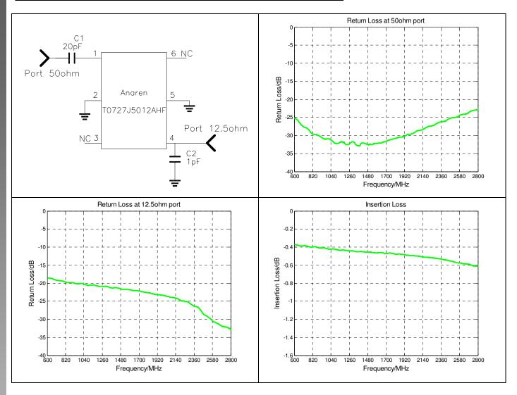
DC connectivity of T0727J5012AHF with pin assignments is shown below. It is noted here that pin1 and pin3 are NC pins without any internal connections, while pin1, pin4, pin 2 and pin 5 are DC connected internally together. To have T0727J5012AHF function properly, pin 2 and pin 5 are required to be grounded by the mounting footprint.
