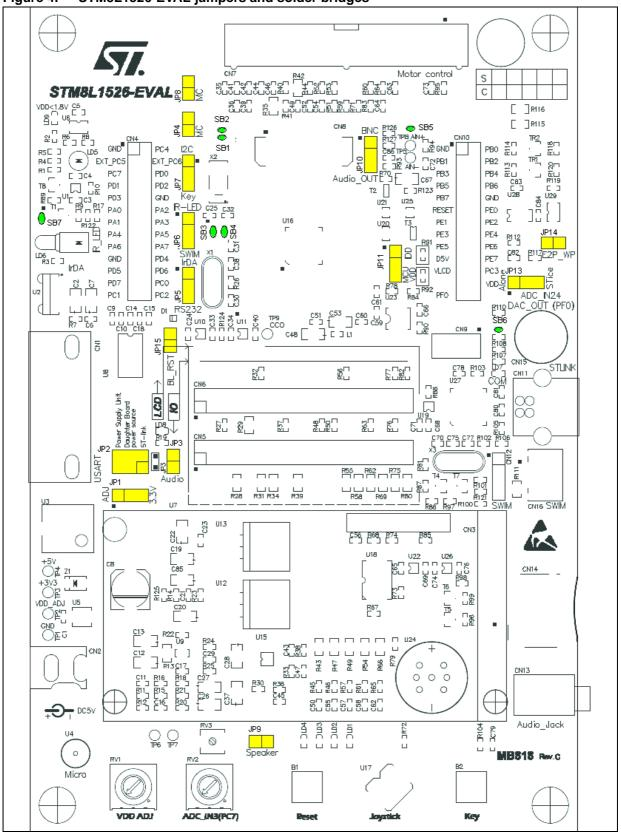
Figure 4. STM8L1526-EVAL jumpers and solder bridges
