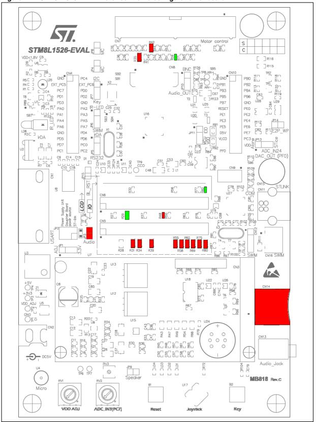
Figure 7. STM8L1526-EVAL motor control re-configuration of board
