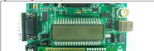
Figure 5. LCD glass module in position I/O
